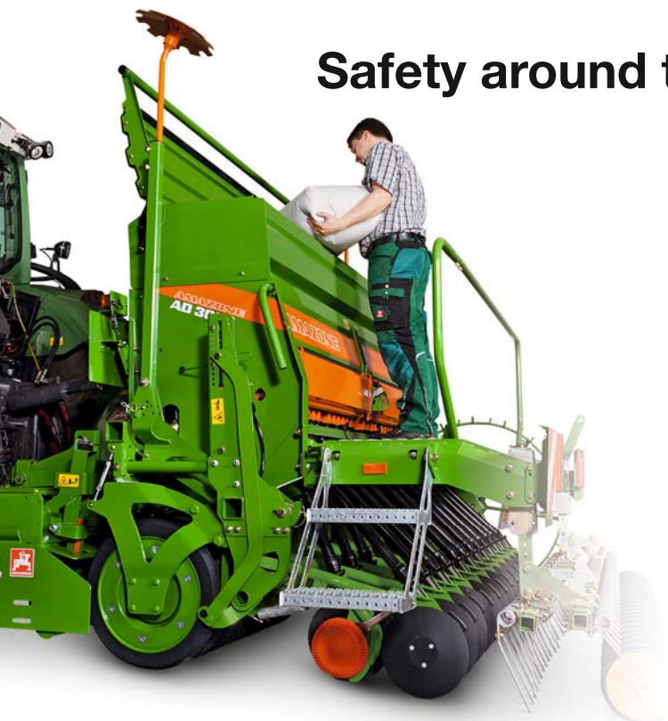
The loading aid helps the filling of the seed hopper when using bagged material.
