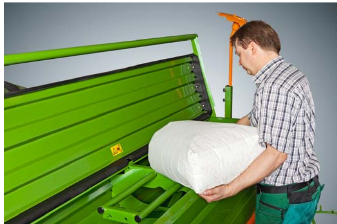
The loading aid helps the filling of the seed hopper when using bagged material.
