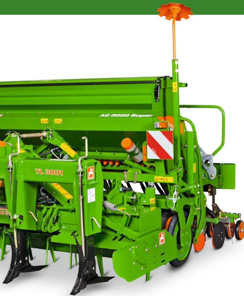
AD pack top seed drill in combination with TL deep loosener, KG rotary cultivator and KW wedge ring roller
