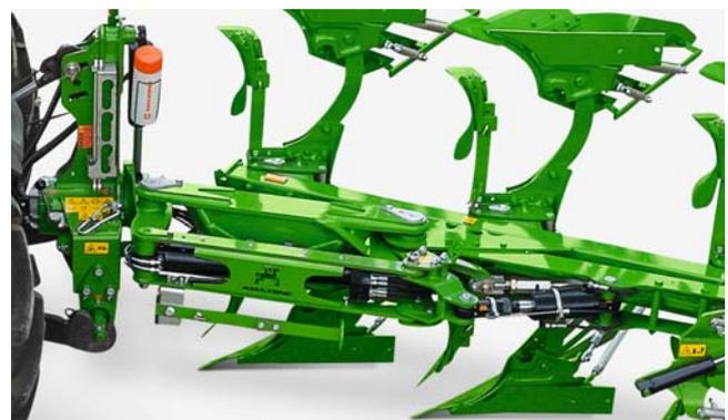
Another special benefit of the Cayron plough is that the beam swivels as standard prior to the turning procedure without any movement in the plough body bearings.
