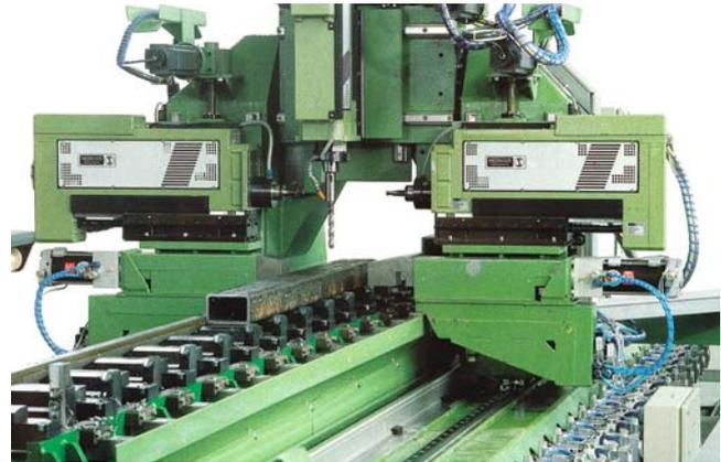
All the beam box sections are drilled out using a specially developed boring process where all the holes are machined out in a single action to ensure the utmost precision in the manufacturing process.
