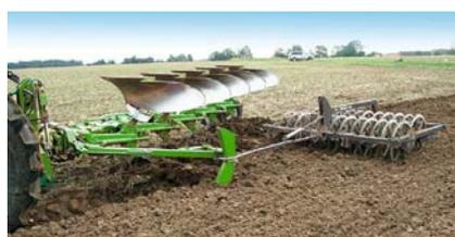
For use in combination with a plough press, all Cayros ploughs can be equipped with a hydraulic, length adjustable press arm.
