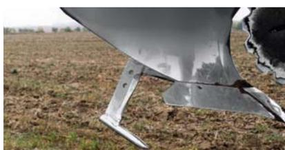
Using the adage 'plough shallow and then deep loosen' the subsoiler points break through the soil layers below the plough depth. The subsoiler points are adjustable in depth and are easily exchanged to keep the running costs as low as possible.
