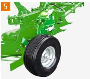
**5** Wheel Ø 680 mm air-filled tyre x 250 mm wide
