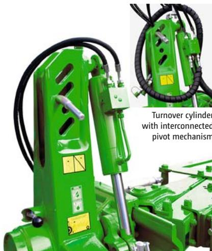
Turnover cylinder with interconnected pivot mechanism
