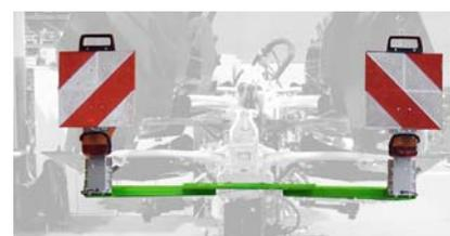
All Cayros ploughs must also be fitted with a lighting kit for road transport. Either pointing to the left (for transport with plough in working position) or double-sided for use with combined transport/depth wheel. The lighting system ensures safety whilst driving on public roads.
