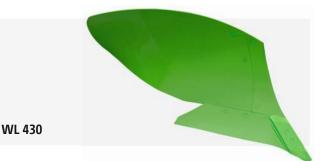
Heavily scrolled and long-drawn for light to heavy soils, outstanding furrow clearance for wide tyres up to 710 mm, best handling of crop residues. Excellent behaviour in sloping terrain. Working depths of 15 to 33 cm.
