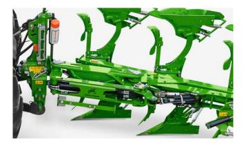
Another special benefit of the Cayron plough is that the beam swivels as standard prior to the turning procedure without any movement in the plough body bearings. This results in much more free space underneath the beam when turning and avoids wear.
