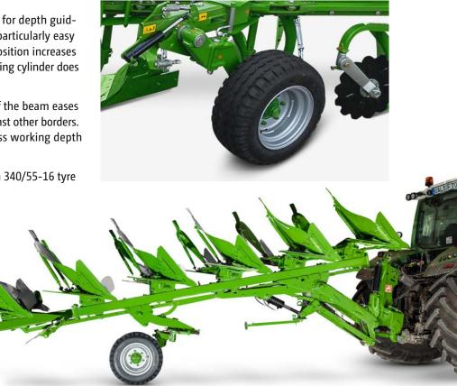
An especially comfortable conversion from work into the transport position by folding round the wheel arm
