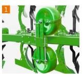
Wheel Ø 500 mm steel x 185 mm wide Suitable for: M & XM ploughs. All beam heights Mounting position: On next to last body for optimum field edge ploughing
