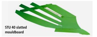
Universally-usable body for light to heavy, but above all, sticky soils. Due to the wide furrow clearance, crop residues are superbly incorporated. The slats can be exchanged individually to reduce the wearing costs. Working depths of 18 to 40 cm.
