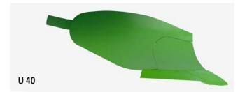
Universal body for light to medium heavy, easy-turning soils. Especially wide furrow clearance and thus good incorporation of crop residues. Very easily pulling with good crumbling. Working depths of 18 to 40 cm.
