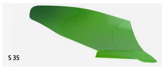
Heavily-scrolled, helical body for heavy marshland and Polder soils. Intensive inversion of the soil furrow. Especially good furrow clearance and cleaning properties. Working depth of 15 to 30 cm.
