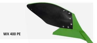
Very shallow, scrolled plough body for very heavy soils. Equipped with a mouldboard made from special plastic resulting in best cleaning properties for extremely sticky soil conditions. Working depths of 12 to 25 cm.
