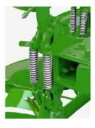
on the Cayros M, an alternative to using either shear bolts or NonStop protection systems when the ground is not excessively stony.
