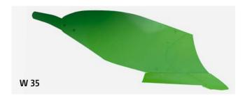
Scrolled body, suited for medium-heavy loam and clay soils. Easy pulling with a simultaneous good furrow clearance and good soil inversion. Working depths of 15 to 30 cm.
