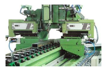
All the beam box sections are drilled out using a specially developed boring process where all the holes are machined out in a single action to ensure the utmost precision in the manufacturing process.
