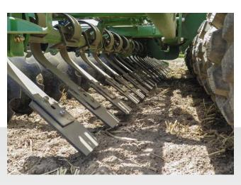
Crushboard in front of the tyres – for distributing and settling the soil
