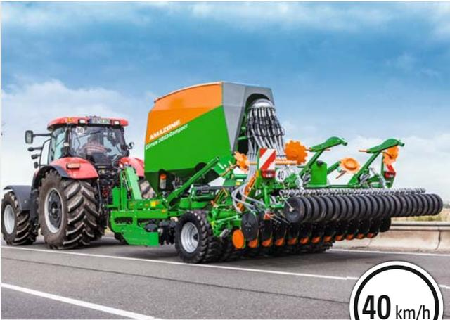
❶ “As standard, the Cirrus is equipped with a very efficient air braking system – exemplary! However better still: equipped with this the machine is allowed, even with a full hopper tank, to travel at 40 km/h on the road.”
