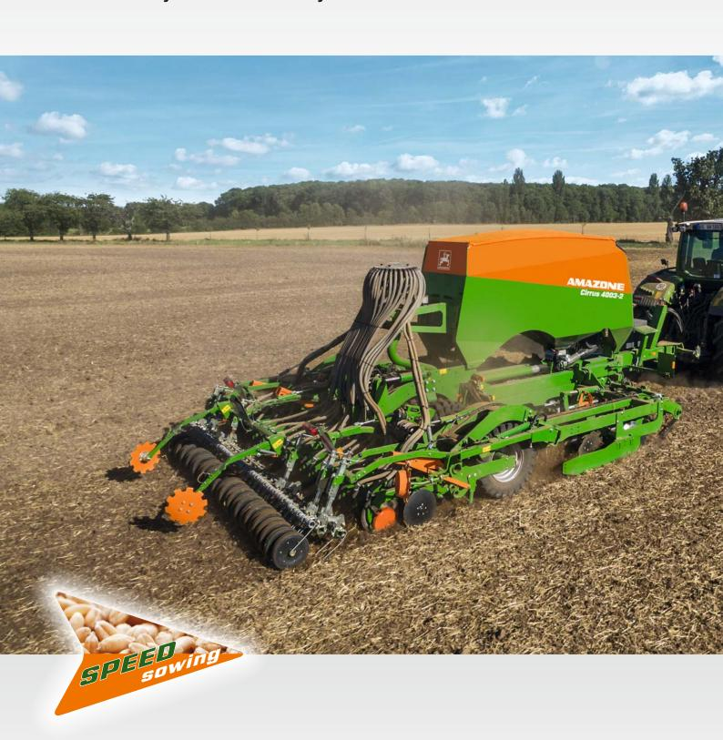
The Cirrus trailed cultivator drill is a pneumatic seed drill which is characterised by its superb working performance; both in conventional and mulch sowing.
