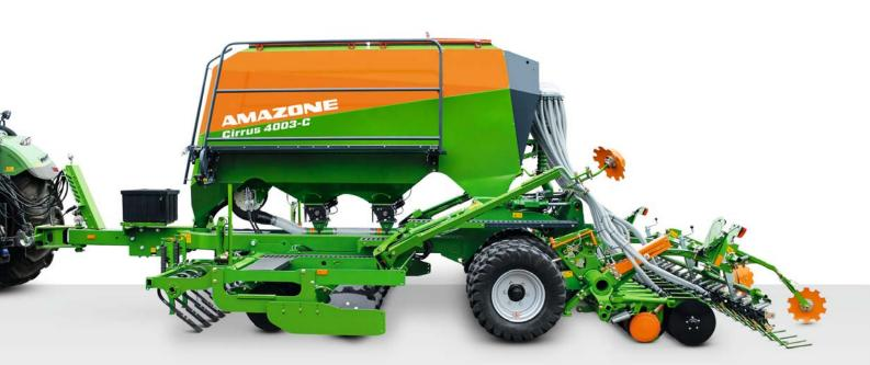
Cirrus 4003-C with twin outlet pressurised hopper for seed and fertiliser
