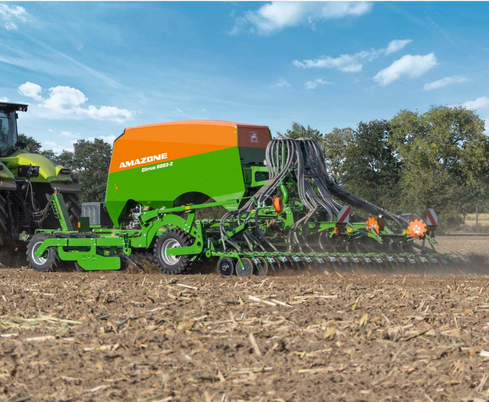
❗ “The shape of the seed tube in the coulter was changed to place the seed even more precisely in the bottom of the furrow. This also functions very well – when the seeds were uncovered we did not find anything left on top. Almost all the seeds were left on the water-bearing seed furrow bottom.”
