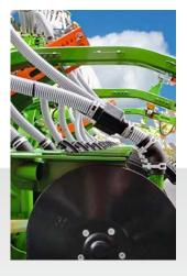
Sensor for registering seed flow at the sowing coulter
