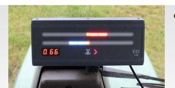
External light bar for CCI.Command.PT parallel driving aid As a possible addition, an external light bar is available which can comfortably be coupled with CCI.Command PT. The external light bar Can be positioned freely in the tractor cab. The only precondition for its utilisation is the activation of the Parallel Tracking module in CCI.Command.
