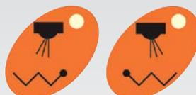
In conjunction with the Super-S boom and either AMASET+ or AMASPRAY+, these press buttons can also be used to control boundary or end nozzle control.
