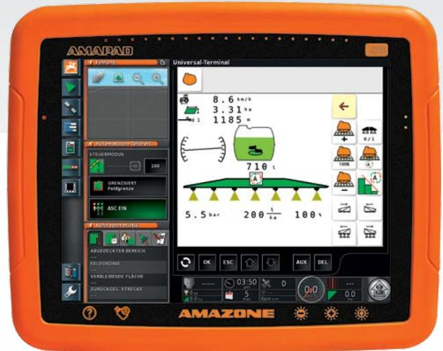
In addition to GPS-Switch pro part-width section control, a high-quality professional manual light bar guidance system is also installed as standard. GPS-Track can also be upgraded to an automated steering system.
