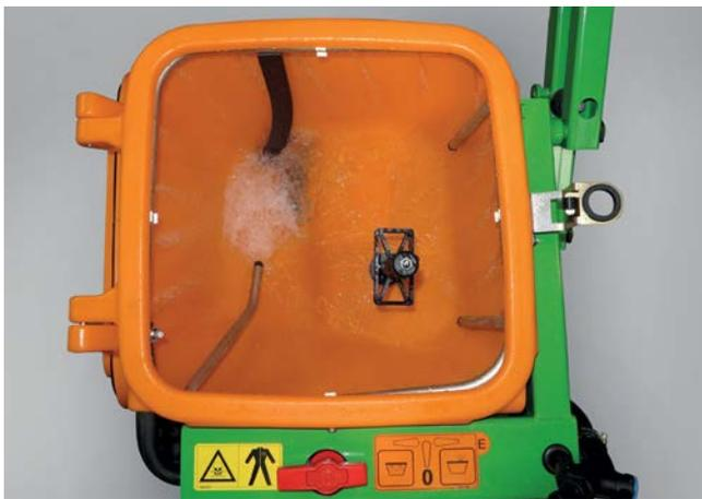
With the Venturi system, a high fill throughput is attained. The same professional induction bowl is used on the UX trailed sprayer.
