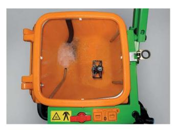
With the Venturi system, a high fill throughput is attained. The same professional induction bowl is used on the UX trailed sprayer.
