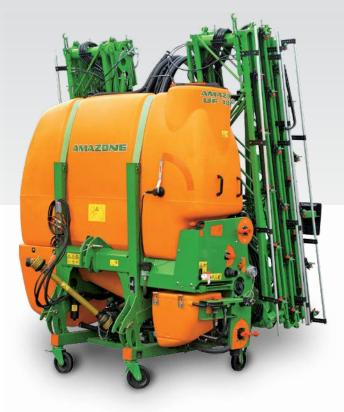
UF 1801 with 24 m Super-S2 boom and transport wheels (braked)
