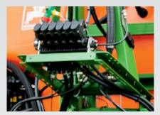
✔ Electrically-controlled TG valve chest For actuation using either ISOBUS or AMASPRAY<sup>+</sup>, modern valve chest technology is utilised. The part-width boom sections are switched, on and off, quickly and drip-free via electric motor valves with pressure relief. In all situations the spray rate is exactly and quickly controlled directly via the computer and so negating the need for any mechanical equal pressure control.
