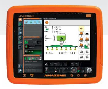
In addition to GPS-Switch pro part-width section control, a high-quality professional manual light bar guidance system is also installed as standard. GPS-Track can also be upgraded to an automated steering system.
