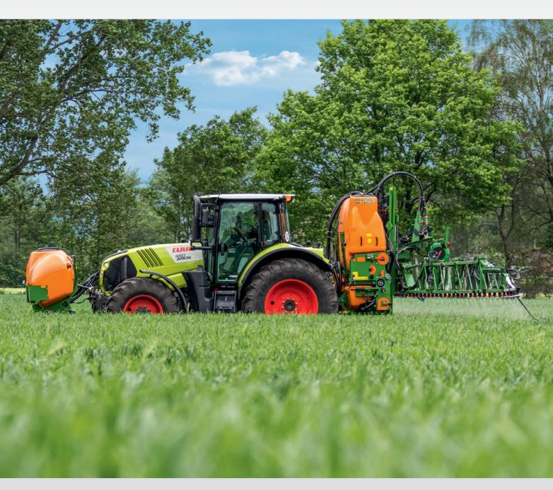
"Due to the intelligent control of the liquid flow circuit, AMAZONE has managed to make the front tank really practical." Via the FT front tank, the tank volume of the UF mounted sprayer can be very simply increased by 1,000 l. Thanks to the optional FlowControl System and the compact design, the UF front tank is the ideal solution for increasing the overall capacity of the UF.
