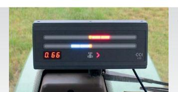
External light bar for CCI.Command.PT parallel driving aid As a possible addition, an external lightbar is available which can comfortably be coupled with CCI Comand PT. The external lightbar can be positioned freely in the tractor cab. The only precondition for its utilisation is the activation of the Parallel Tracking module in CCI.Command.
