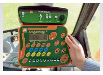
With the AMASPRAY<sup>+</sup> in-cab terminal in combination with Proficlick, the sprayer can be comfortably operated."
