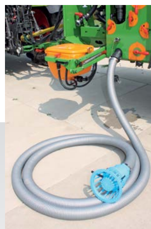
Filling via the suction hose
