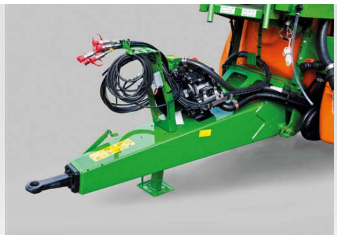
AutoTrail axle steering with rigid straight drawbar or rigid hitch drawbar in the field.
