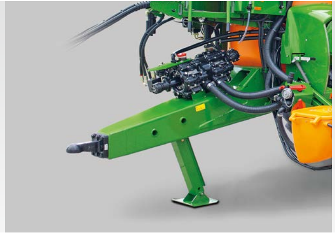
Hitch drawbar, rigid with hydraulic pump drive
