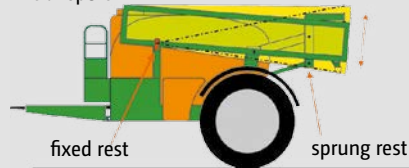
Sprung damping of the boom during transport
