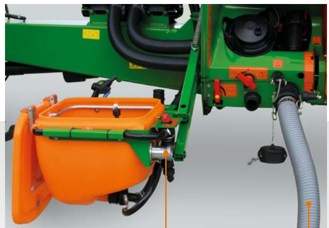
Ecofill with rinsing pedestal – clean filling from large containers
