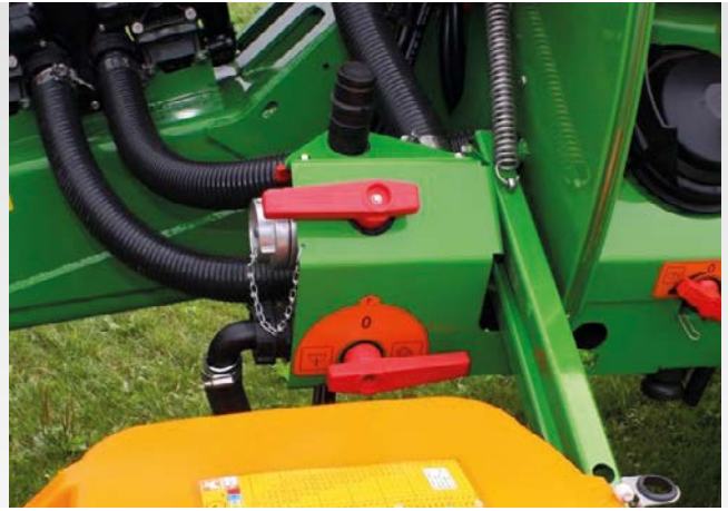
Switching on the injector enables fill capacities of up to 700 l/min (UX Super) and 500 l/min (UX Special).
