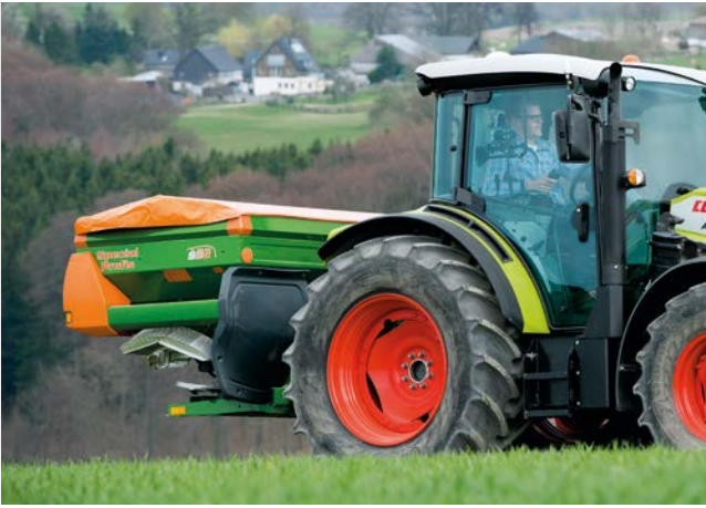
ZA-M 1001 Special Profis weigh-cell spreader with right hand Limiter in normal spreading position
