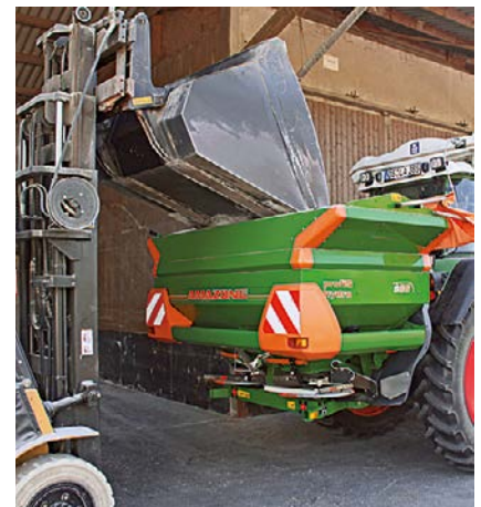
Filling with a loading shovel
