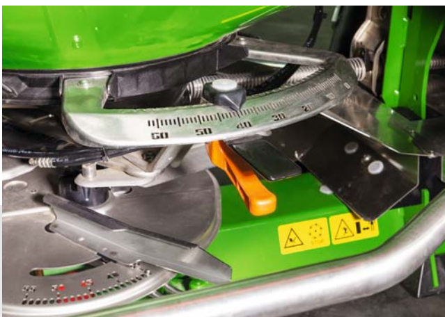
Setting lever with large scale
