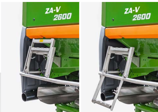
Foldable ladder for the ZA-V with S 2600 extension
