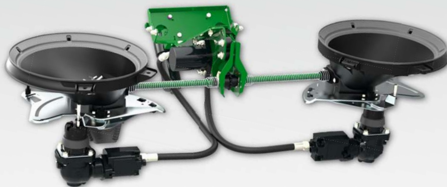
Schematic representation of the hydraulic drive on the ZA-V
