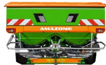
S 2600 extension (filling width 2.22 m) with foldable ladder on left hand side
