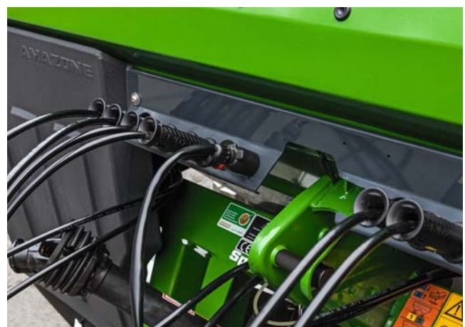
Accessible holder for the hydraulic hoses
