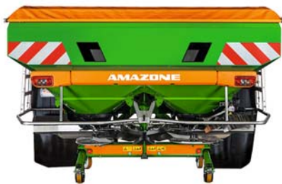
L 3200 extension (filling width 2.71 m) with foldable ladders
