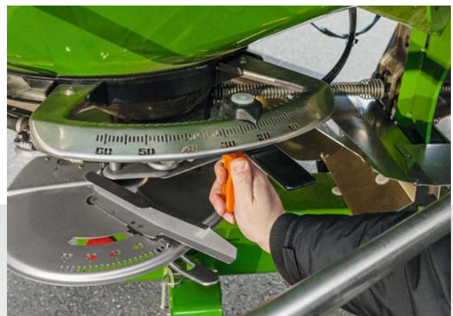
Simple adjustment of the shutter slide assembly
