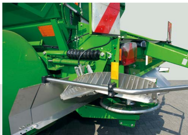
Limiter border spreading system raised out of work
