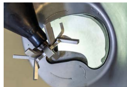
Stage 3: Hopper aperture wide open
