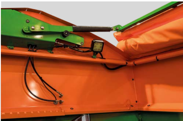
Work lights inside the hopper
