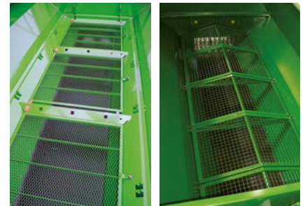
Large protective sieves – the spreading system is optimally protected from stones or other foreign objects.
