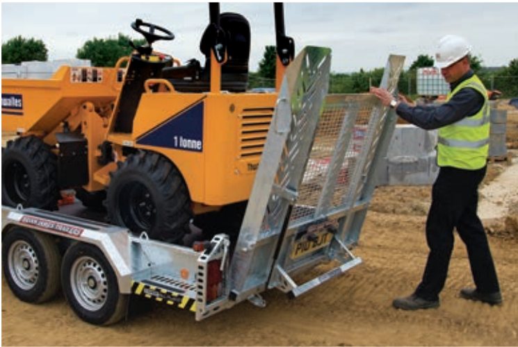
Easy ramp operation with gas spring assistance, enables opening and closing with less effort.
