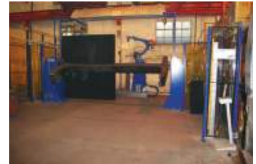
Above: New Robotic Welding Cells
