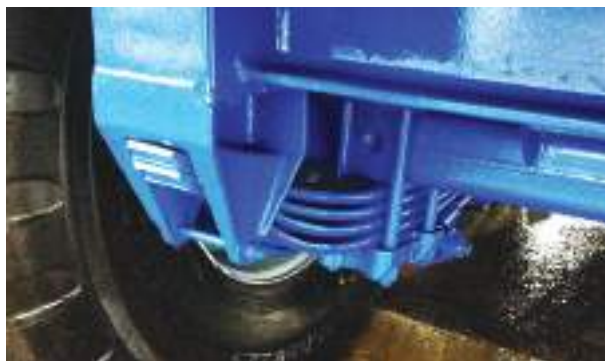
4-leaf Parabolic Springs
