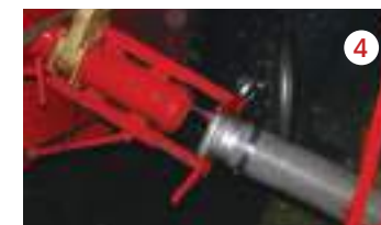
Once the tanker has filled, the operator extends the connection fork and reverses away from the hose before retracting the connection fork and driving away.
