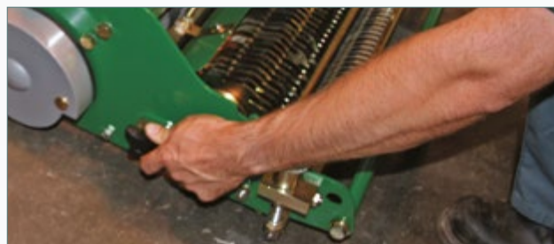
Loosen retaining bolt and slide cassette across
