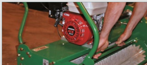
Lower cassette onto back tie bar and slide cassette across
