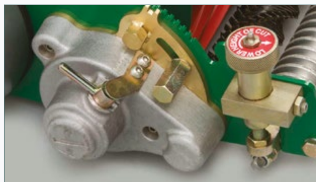
Simple to operate groomer drive engagement
