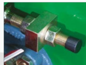
Adjustment of cylinder to bottom blade with a single spanner
