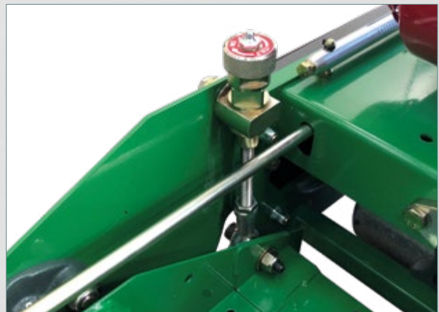
Simple 'click adjustment' for angle of deck
