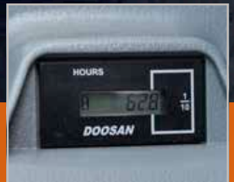
Hour meter (from ground level)
