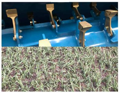
When you replace your "L-shaped" fraising blades with special hybrid chisels, you are enabled to fraise mow the natural grass and surface layer of a hybrid-grass pitch, without damaging the remaining synthetic fibres on the pitch.
