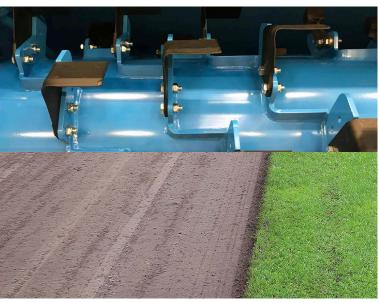
With the Combinator you are in possession of a multifunctional fraise mowing machine. The Combinator is equipped with the CombiRotor®. You can provide the CombiRotor® with three distinct types of blades or chisels. In order to fraise mow the surface layer of your natural grass sport pitch, you are required to assemble the "L-shaped" fraising blades.
