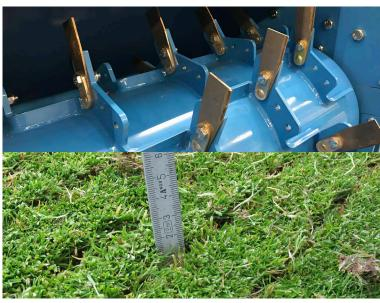
Furthermore, you can also use the Combinator to scarify when you assemble the CombiRotor® with tungsten-carbide scarifying blades. By means of the patented pendulum system of the conveyer rollers, you can easily control the working depth of the Combinator.
