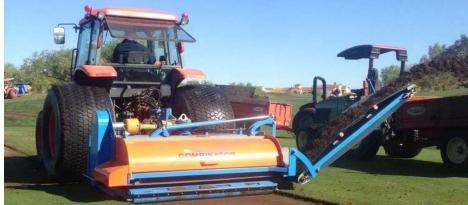
You can directly transport the removed infill material by means of conveyer belts. We have provided the conveyer belts with unique conductors, consequently the conveyer belts will not yield to heavy loads.
