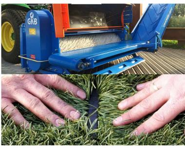
Besides the variable possibilities to operate the Combinator in your natural grass pitches, we also provide the possibility to assemble a specialized brush for synthetic turf in the Combinator. This will enable you to remove sand, cork and rubber (infill). Subsequently, you can separately dispose the removed material.
