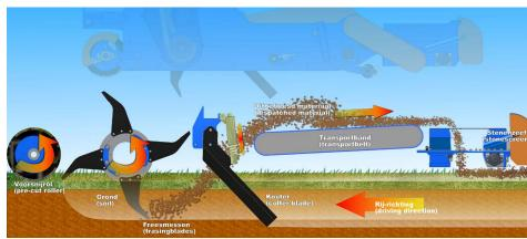
The Ecodresser is equipped with a cutting roller, which ensures minimal operating damage to the turf. The hook tines extract the dressing soil form the present upper layer, these hook tines are equipped with slipping. The coulters, which ensure the aeration of the upper layer, are spring-loaded. In order to prevent damage from stones in the pitch.
