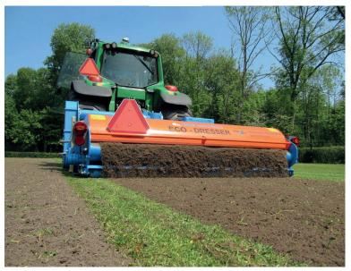
With the Ecodresser you are is possession of the ultimate machine for the maintenance of your sports pitches or golf courses. Multiple operations are combined. The turf is intensively aerated (20 cm deep). At the same time the dressing is applied to the surface layer and the sub layer is aerated. Subsequently, it is possible to level the imperfections.
