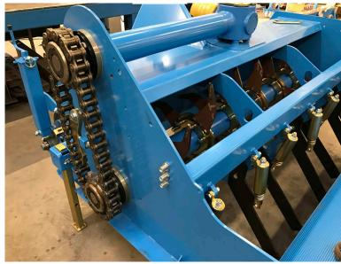
The rotor that is positioned in the Ecodresser, is delivered with a slipper clutch. Thus, you can operate the Ecodresser on rough terrain. Furthermore, we assemble the Ecodresser with sprung coulters, these ensure the aeration of your pitch.
