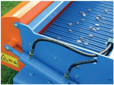
You can level imperfections in your pitch by carrying the recycled dressing soil on the conveyer belt, following you can scatter it on the desired area of the pitch. There is an option to equip the Ecodresser with a stone screen and collecting tray, in this way you are able to create a homogeneous upper layer.
