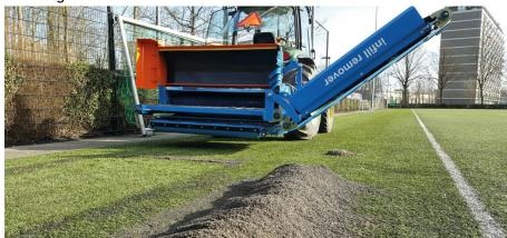
The Infill Remover works with an unique brush. You have the possibility to adjust the stiffness of the brush. As a result it is possible to work on both new pitches, as well as on heavily compacted pitches. Depending on the characteristics of the pitch, it is possible to remove the entire layer of infill in jsut one operation.
