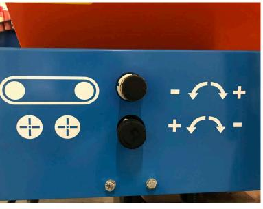
As standard, the control unit of the conveyor belt and the spreading discs, is mounted on the Sandspreader. Nonetheless, we provide the option to deliver the Sandspreader with a touchscreen, that will allow you to control these functions from the cab of your tractor. Moreover, a conveyer belt on the front will enable you to use the Sandspreader as a buffer machine.
