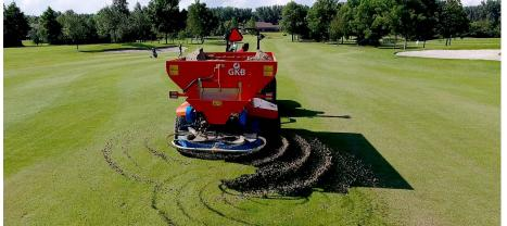
The shape and design of the sand bunker ensures an efficient operation and ensures your clear view along the machine. The sand is transported to a metering valve by means of a conveyer belt, which, optionally, is also available as a hydraulically operated metering valve. The double, hydraulically powered, spreading discs are adjustable on multiple points, consequently, the Sandspreader enables you to create perfect sand distribution.
