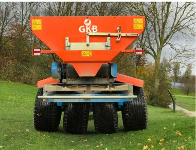
Accordingly, we can deliver the SP100 with a wheel set containing four pivoting balloon tires. All other Sandspreader models are delivered with four pivoting balloon tires as standard, in order to assure the perfect weight distribution on your sports pitch or golf course.
