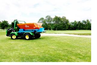
The Sandspreader is available in four distinctive designs. The capacity of the bunker varies from 1 m3 to 4 m3. The SP100 is suitable for assembling on a turf truck. For instance, on a ProGator, Truckster or Workman.
