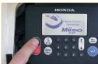
A clear and easy to use control panel which allows you to change Miimo's functions and set a security code
