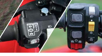
With it's automatic clutch, ESP lets you quickly and easily shift between gears with a pair of handlebar mounted buttons, for added convenience in tough, muddy conditions.
