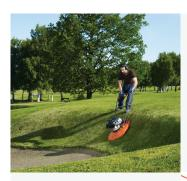
**Cuts on slopes up to 45°** Cuts continuosly on slopes up to 45° due to the oil throw engine lubrication system.
