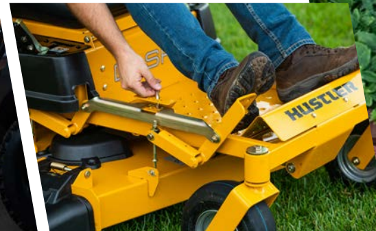
Lift the deck easily with foot-operated mechanism.
