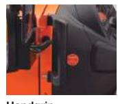
**Handgrip** For easier entry and exit, all new B1 Series models feature a handgrip on the left side.
