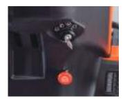
Engine Key Stop A 4-position (preheat/on/off/ start) key-operated switch operates a solenoid to shut off the engine.
