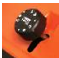
Easy reach cutting height adjustment dial
