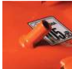
Deck cleaning pipe for connecting water hose
