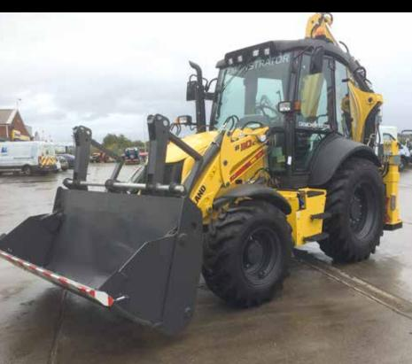
The New Holland backhoe range can be equipped with a wide choice of buckets to match excavation, water course clearance, trenching and other demands. Post hole borers, hydraulic hammers and countless other tools can all be fitted. The long reach of both the standard and telescopic dipper, up to a massive 6,529mm, allows long reach and digging depth comparable to many conventional dedicated excavators.
