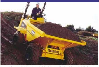
**Engine:** Yanmar 3TNV88, 24.8 kW/33.2bhp (nett) at 2800rpm, 3-cylinder water-cooled direct-injection diesel. Max torque 111Nm (82 lbf ft). Electric starting, hour meter, battery isolator switch and heavy-duty cyclonic air cleaner positioned within the lockable engine compartment.
