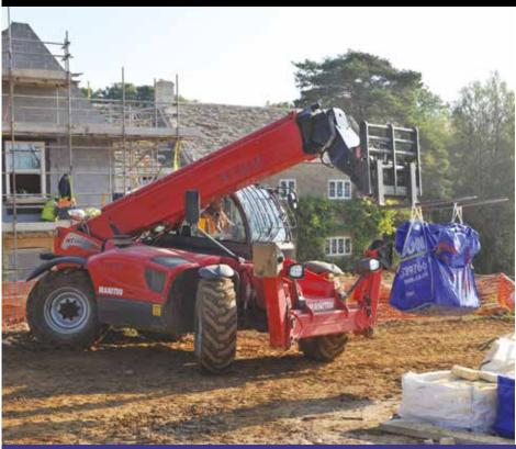
The MT 1440 A telehandler is a great fit for high bay and high rise work sites where a work platform is required to carry out tasks such as roofing and siding. Able to handle 4t loads up to 14m in height, this machine is at home on any type of terrain thanks to its frame levelling system and four-wheel drive and steering.
