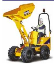
Engine: Yanmar 3TNV76, 15.9kW/21.4 bhp (nett) @ 2800rpm, 3-cylinder water-cooled diesel. Max torque 66.4Nm (49 lb f ft). Electric starting, hour meter, battery isolator switch and heavy-duty cyclonic air cleaner positioned within the lockable engine compartment.
