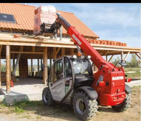
The MT 625 H telehandler is specially designed for building sites and renovation projects involving lower heights.
