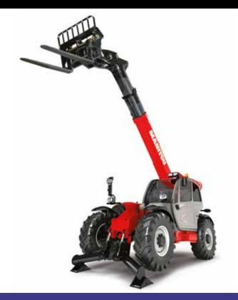
The MT 1135 is a specially-designed telehandler for work sites in buildings up to two/three storeys tall. It comes equipped with a 102hp motor and in terms of performance offers you a lifting height of up to 11m, with compact outriggers so you can work in more confined spaces.
