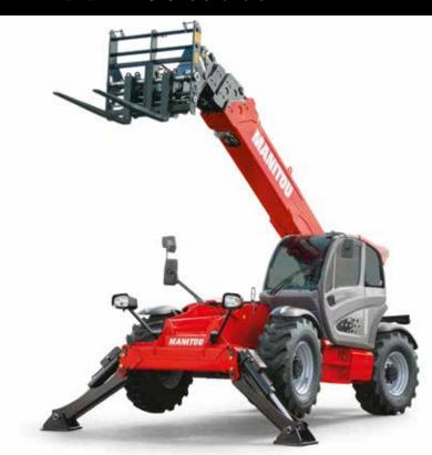
The MT 1840 telehandler is specially designed for high bay/high rise work sites, with a lifting capacity of 4t up to 18m in height. Equally at home on uneven terrain, it has a generous ground clearance and tight turning radius so manoeuvrability never becomes an issue. In addition, excellent lateral and front stability make it a reliable on-site partner.
