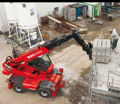
The MRT Easy Rotating Telehandler range is a perfect fit as both your first piece of construction equipment or as part of a rental fleet. Incredibly versatile, it's used for a wide range of applications thanks to the diversity provided by the compatible attachments available (forks, lifts, platforms, crane, etc.) ...a true 3-in-1 machine.
