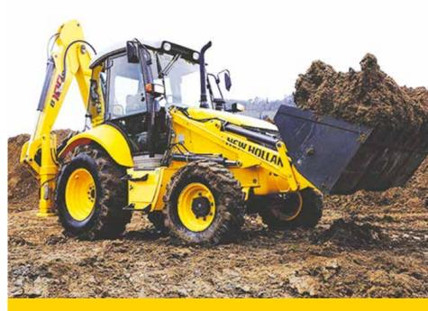
The 4.5 litre turbocharged engines for the new machines are provided by FPT Industrial, a world-wide leader in the design, production and sale of powertrains for industrial applications, supplying among others Fiat Industrial brands such as New Holland Construction and Iveco. The Variable Displacement Pump hydraulic system is standard on B100-B and above, contributing to a 10% fuel saving and a rapid return on investment.
