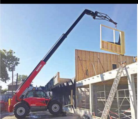
The MT 1335 is designed with work sites up to two/three storeys tall in mind. It comes equipped with compact outriggers which improve its offset as well as the general performance of the machine as it can easily navigate more confined spaces. Its lifting capacity is 3.5t up to heights of 13m. And for the comfort of the operator, the spacious driver's cab is equipped with the JSM system and an ergonomic, intuitive instrument panel, and is easily accessed with its wider door.
