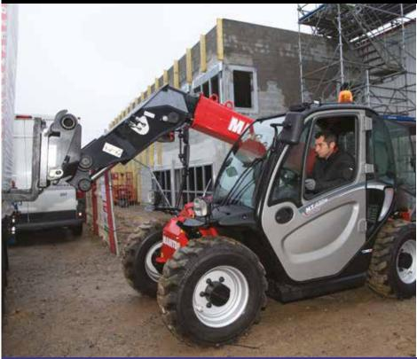
The 420 H New Buggy is the most compact telehandler in the MT Manitou range. With its exceptional dimensions, the MT 420 H New Buggy is the ideal partner on any worksite. Capable of negotiating the most confined, uneven and difficult-to-access spaces, the MT 420 H New Buggy boasts four drive wheels and a turning radius of less than three metres. Enjoy a compact, easily manoeuvrable machine which will help reduce your Total Cost of Ownership.
