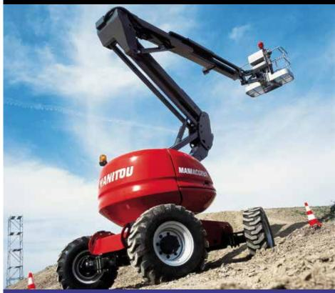
The Manitou articulated platform range is the most suited to work outdoors on uneven or sloping ground. The 160/180/200 models offer capacities of 230kg, up-and-over clearances of 7.38m and working heights of up to 20m, which provide the operator with a large working area.
