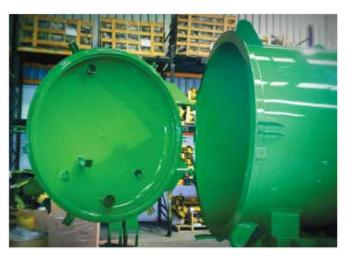
**Fully Opening Rear Door:** These doors are mounted on hinges. They are locked by six threaded hooks.
