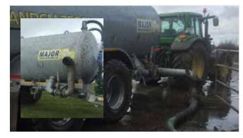
**Autofiller:** 6" or 8" hydraulic coupler. It is ideal for slurry pits that are difficult to access. It reduces your filling time by half. A galvanised tripod is supplied as standard.
