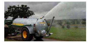
**Raingun:** Centre mounted or rear mounted in conjunction with a garda pump fitted with stone trap as standard.
