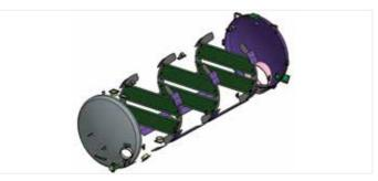
Internal baffle plates improve operator driver safety by preventing wave motions during transport.
