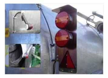
**Double LED Lights:** Double LED lights and LED side markers can be fitted for increased operator safety
