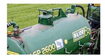
**Top Fill:** The hydraulically controlled top fill is used to fill the tank from the top. This option allows for high flow rates and fills the tank to its optimal level.
