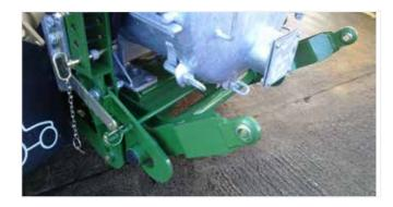
**Rear Linkages**: Linkages can be added to your tanker to allow slurry injector units to be fitted at a later stage.
