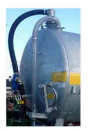
**Full Length Sight Tubes:** To allow the operator to easily identify how much liquid remains in the tank.
