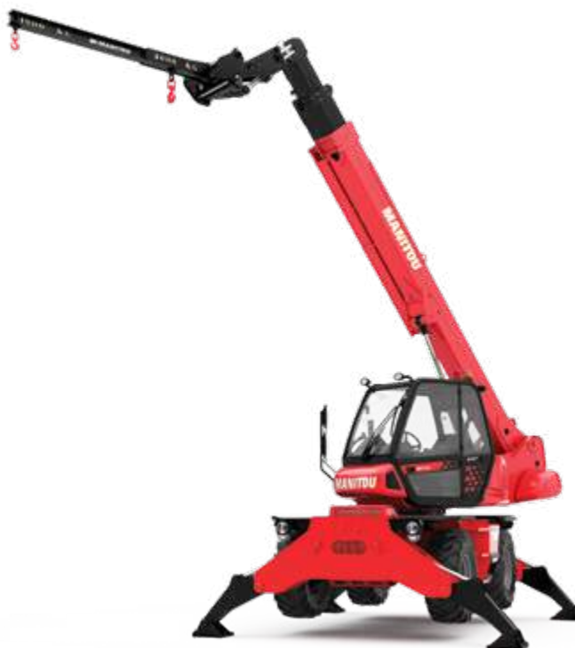
Rotation on lowered stabilisers with 1500 kg jib
