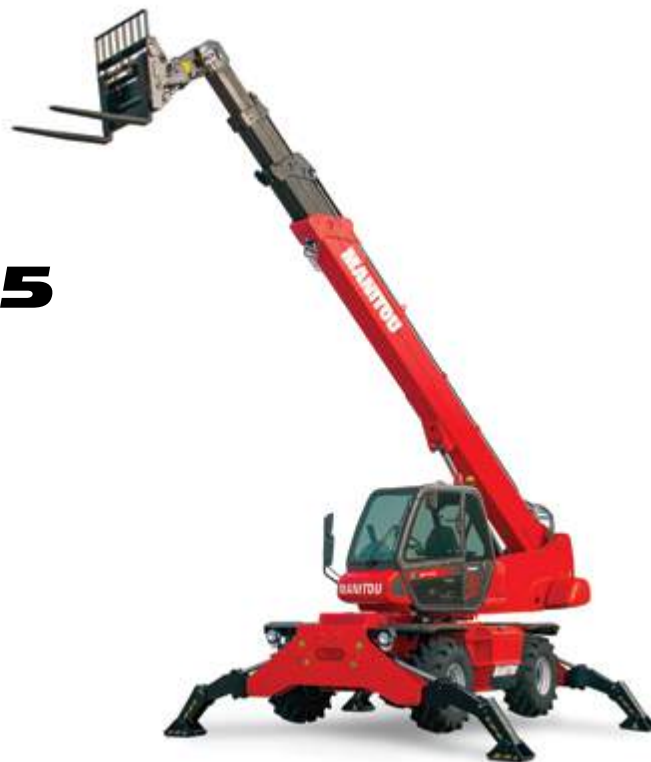
Rotation on lowered stabilisers with forks
