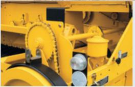
Producing high quality bales day after day, season after season requires robust and reliable drive lines. The dimensions of the shafts, chains and gears as well as the quality of the steel, reflect New Holland craftsmanship and experience. To prevent the buildup of stress on the functional components, the overall baler construction includes a draw bar that is directly connected to the baler axle. Furthermore, a "power pivot support" for the three-joint PTO allows sharp turns with maximum safety.
