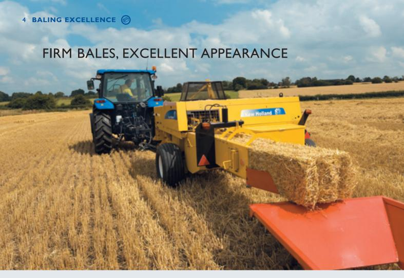
Producing consistent firm bales is a major benefit of the new BC5000 balers. The long bale chamber, allowing for a long plunger stroke, combined with the high plunger speed, ensures a 1<sup>st</sup> class quality bale formation. Adjustable top and bottom bale chamber rails and adjustable bale case doors allow for a perfect setting of the required density.
