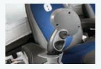
Shift button and ground speed unlock (behind).
