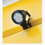
• Rear lamps enable operators to monitor residue and two lamps located on the side panel illuminate the rear axle to prevent crushing standing crop and to assist when manoeuvring
