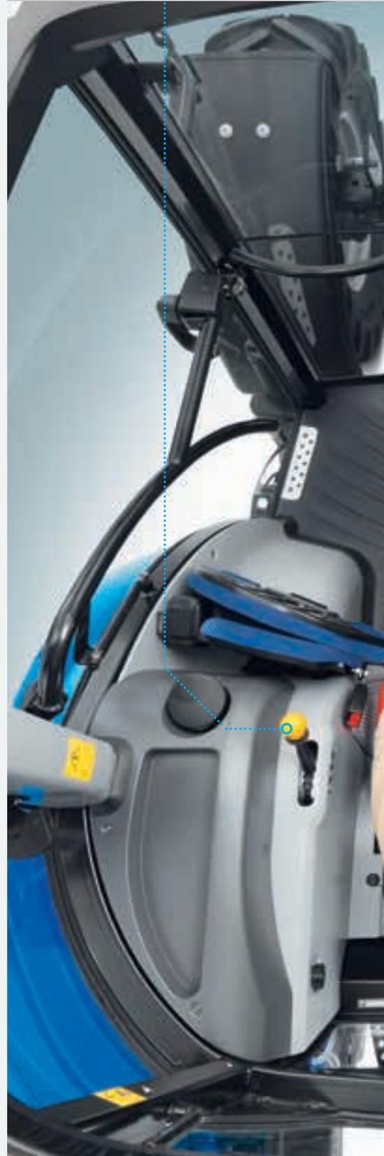
The clear visible instrument cluster moves in conjunction with the fully tiltable steering column, which means you will always have an unobstructed view of key operating parameters. Want to know your PTO speed or even when your next service is due? Simply glance at the easy to read LCD display and you'll be in the know.
