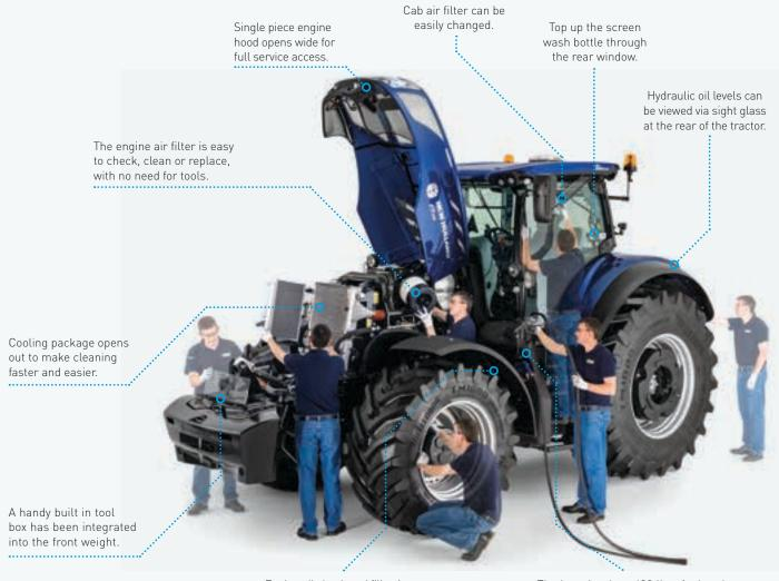
Engine oil check and fill points are easy to reach, with no need to lift the hood. This makes routine checks faster and servicing simpler. The best-in-class 630 litre fuel tank (T7.290 and T7.315) means you can work the whole day long and well into the night without the need to refuel. True 24 hour productivity courtesy of the T7 Heavy Duty range.
