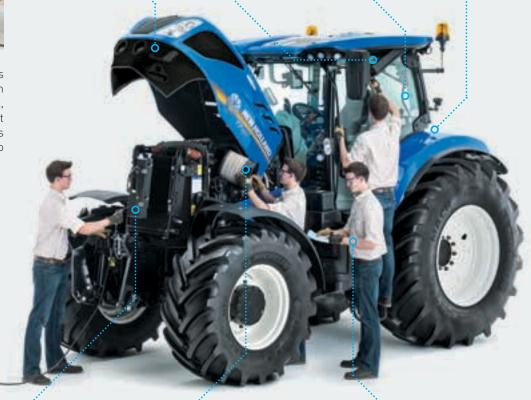
Cooling package opens out to make cleaning faster and easier.
