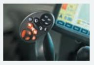
The soft-touch buttons feature backlight technology to make selecting controls in the dark even easier.
