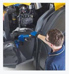
• For security, the 246 litre fuel tank and 37 litre AdBlue tank are accessed only by raising the engine hood
