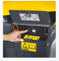
• Hood switch, kill switch and remote battery terminals are grouped at the rear
