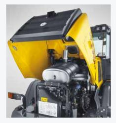
• One piece engine hood features electric opening on W130 D and W170 D models
