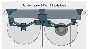
Longitudinal linkage Compensator arm Parabolic spring
