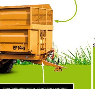
Front inspection ladder, body drain plugs and body prop are standard on all SF and RC models. Perspex window and arched front window options are available.
