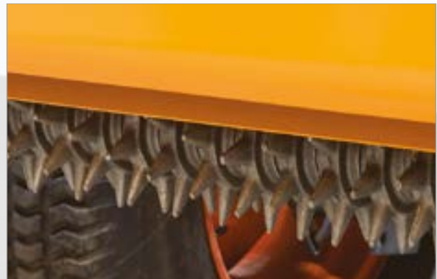
Studded roller for minimal surface disturbance and creating the seedbed 'plant pots'
