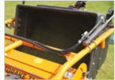
Large capacity collection box, shown with optional hydraulic tip kit
