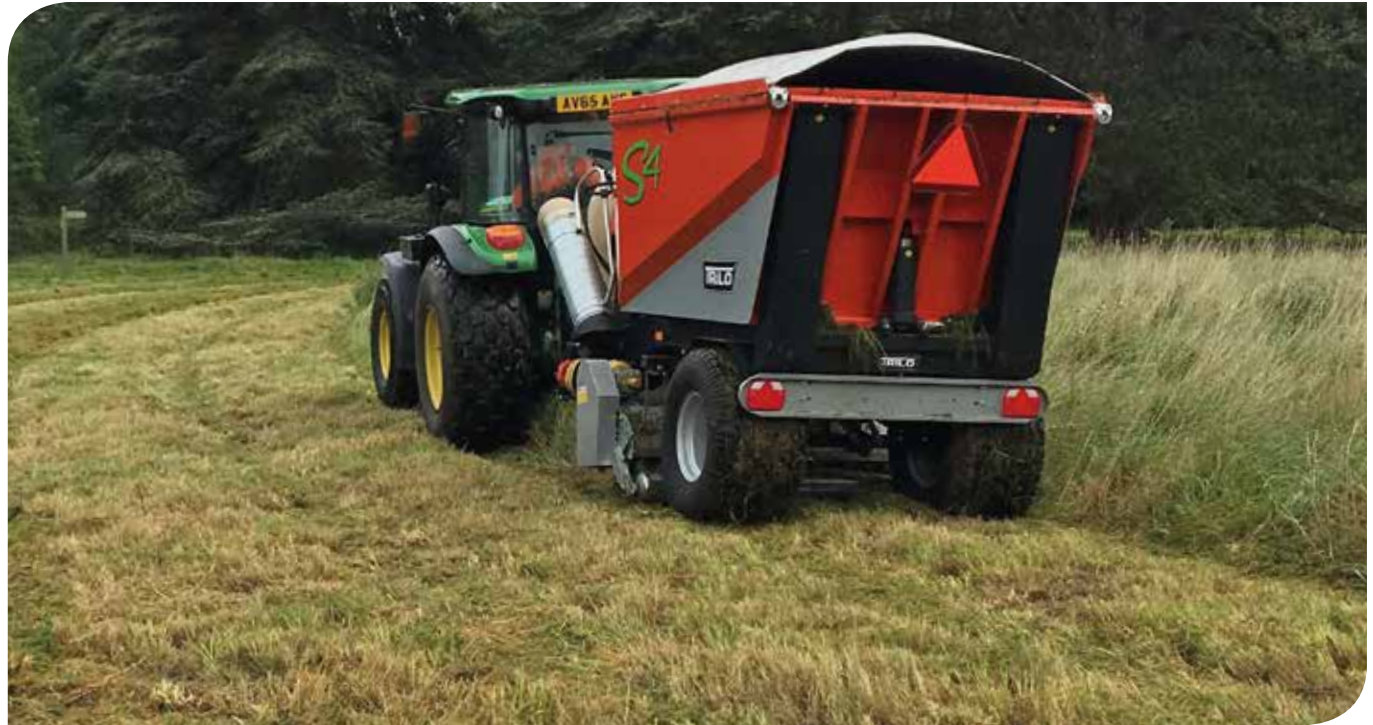
Mowing and collecting high grass on coarser areas is no problem for the S4 vacuum sweeper
