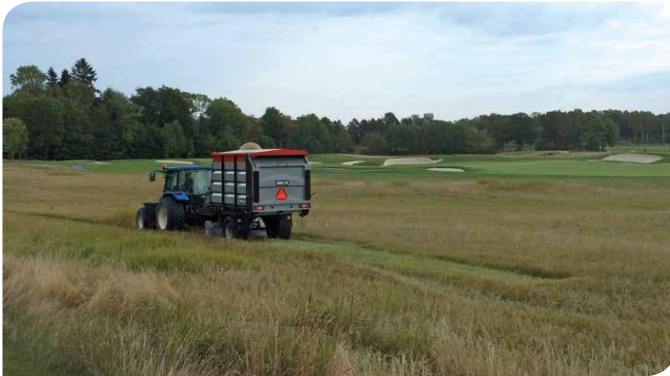
A TRILO® S8 Multi-Purpose vacuum sweeper mows and collects the rough in one pass
