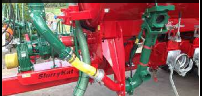
Tankers with DODA Pumps
