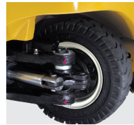
Extended steering axle for class leading manoeuvrability
