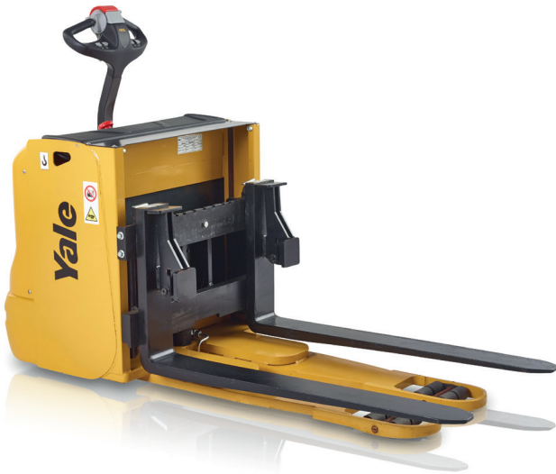
MS24HBE showing raising and lowered battery stops.
