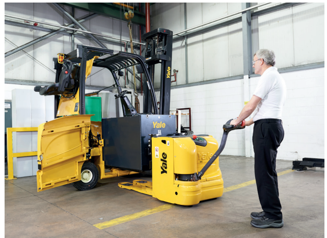
MS HBE powered battery side extractor
