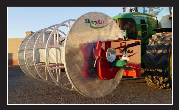
To unhitch the spool there is just one pin for the operator to remove after the tractor's linkage has been lowered to the ground.
