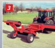
Swing the side section into working position
