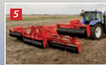
Outside wing cylinders extending
