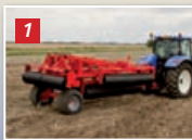
Rolls in transport position, wheels down
