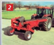
Lift wings off transport cradles
