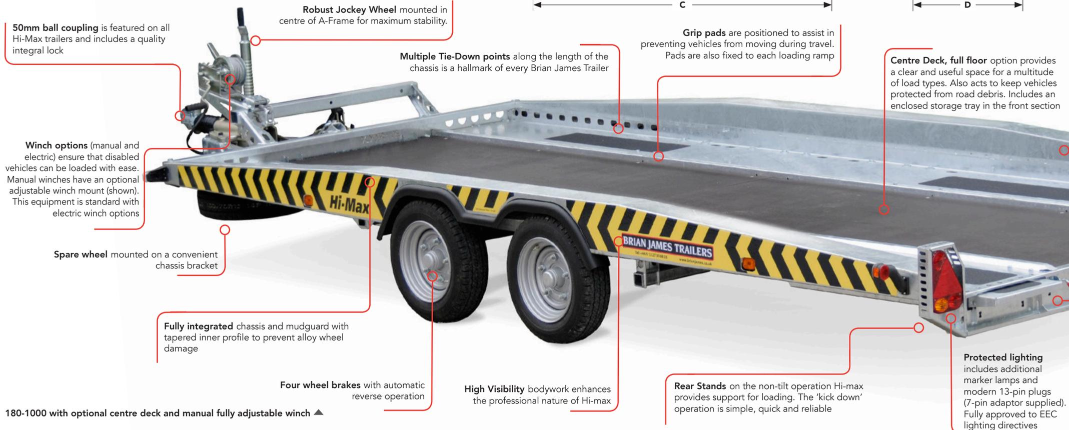
180-1000 with optional centre deck and manual fully adjustable winch ▲
