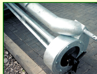
External fins break lumps and force feed the impellor for high outputs.
