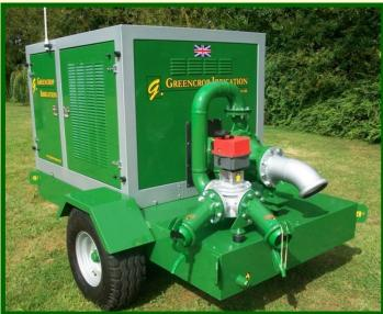
Two models, the GCEP125S and GCEP170S using lveco N45 125HP and N67 170HP engines, encompass purpose designed engine and pump management systems to allow for either automatic pressure maintenance, enabling the operator to specify a required pump outlet pressure where the controller will modulate the engine speed to maintain the required pressure, or remote throttle control via radio telemetry. All Greencrop controllers include full engine protection and auto start facilities.
