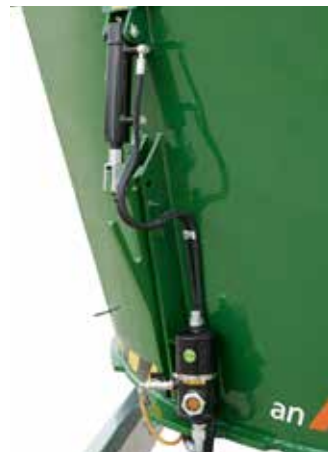
Counterknives to aid chopping and mixing (hydraulic optional)
