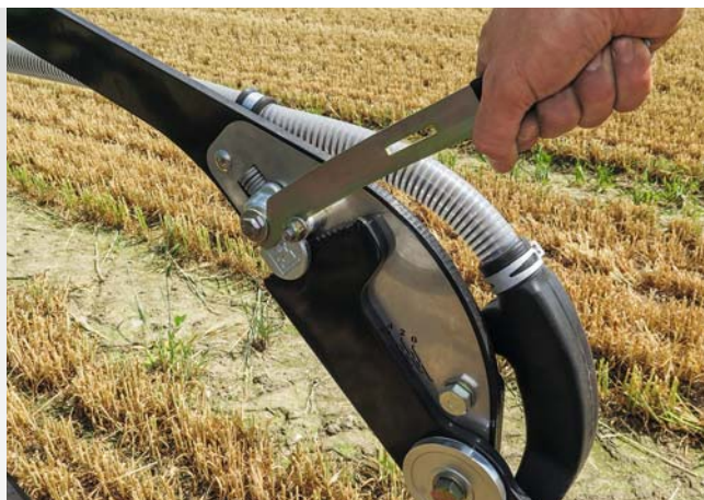
Setting the depth guidance on the tine coulters
