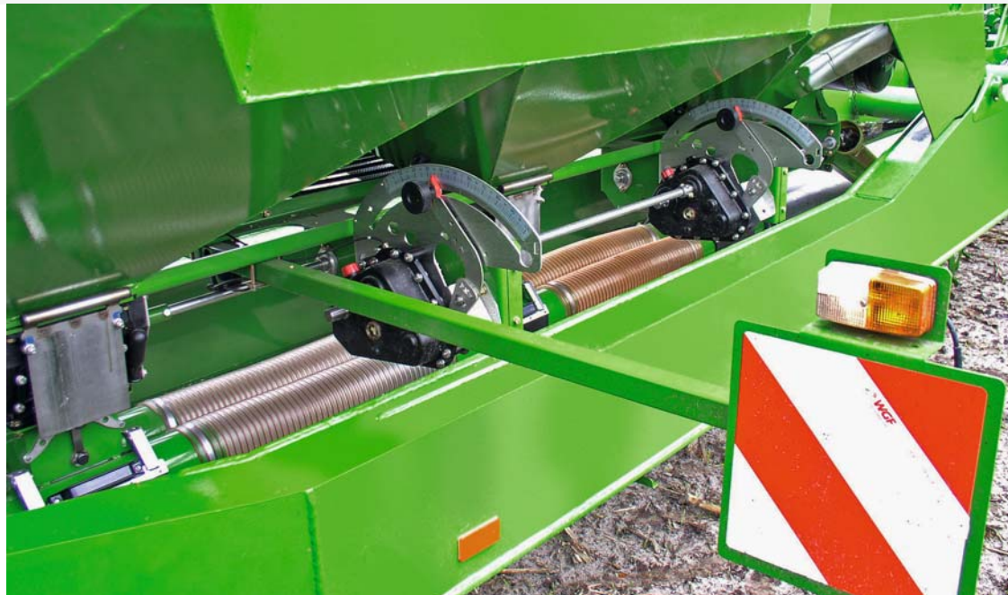
The Vario gearbox provides seed rates of 2 to 400 kg.
