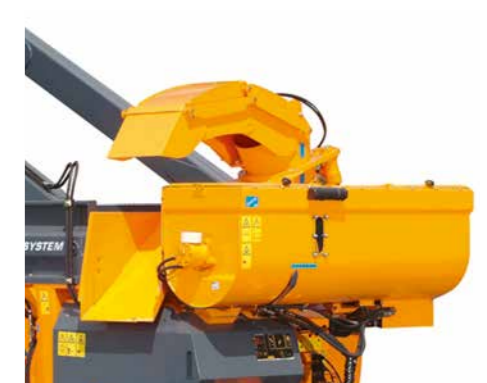
500 L Mixing Hopper System that integrates dry nutrients that will be distributed with the silage
