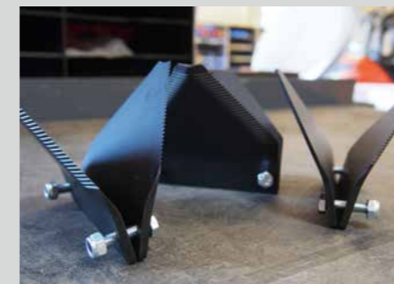
Curved cutting knives to preserve the abrasiveness of the shredder
