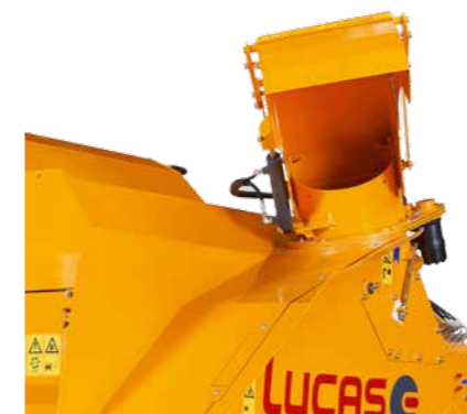
Swivelling chute - 270° Straw blowing 15m right side / 13 m left side
