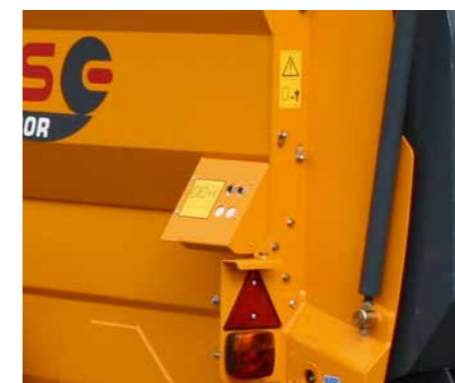
2nd control unit Control of rear collection door to save time when loading.
