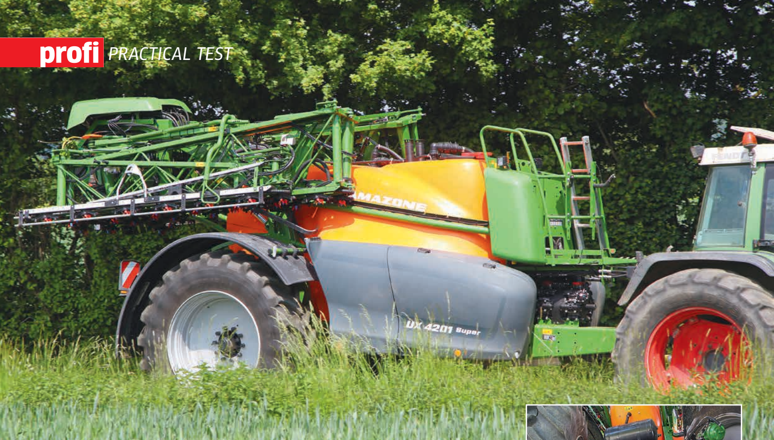
The Super L boom swiftly folds into a compact package. Load-sensing brakes and a 12.5t gross weight allow you to travel at 60km/hr even when filled with ammonium nitrate urea solution.
